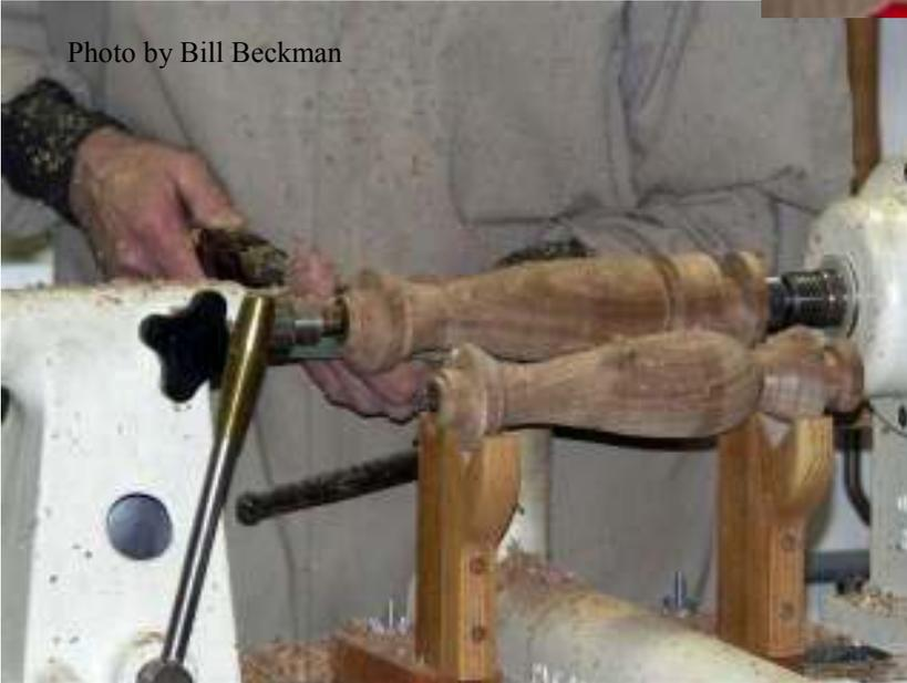
Duplication for furniture, the last third of the presentation, was oriented around a pair of spindles that were part of a butter-nut and glass shelf project. The story pole, the parting tool, and calipers were introduced here.
