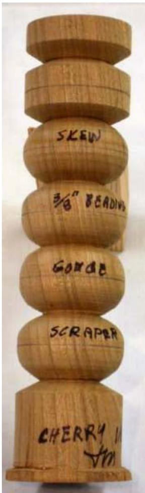
The beads to the left can be “rolled” with almost anything. A skew gives the best surface, but not much better than a sharp gouge. The shape just above the skew-rolled bead is a cylinder flanked by grooves made by my skew. This creates room for the bead rolling.
