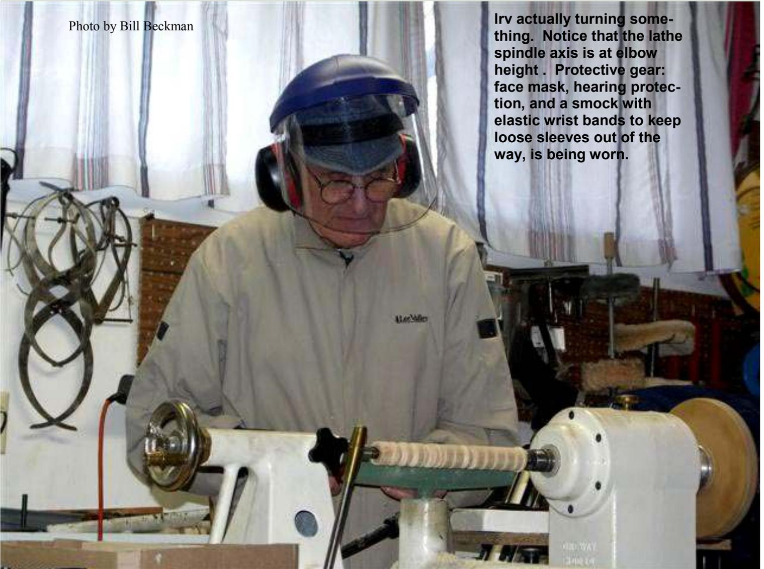
Irv actually turning something. Notice that the lathe spindle axis is at elbow height. Protective gear: face mask, hearing protection, and a smock with elastic wrist bands to keep loose sleeves out of the way, is being worn.
