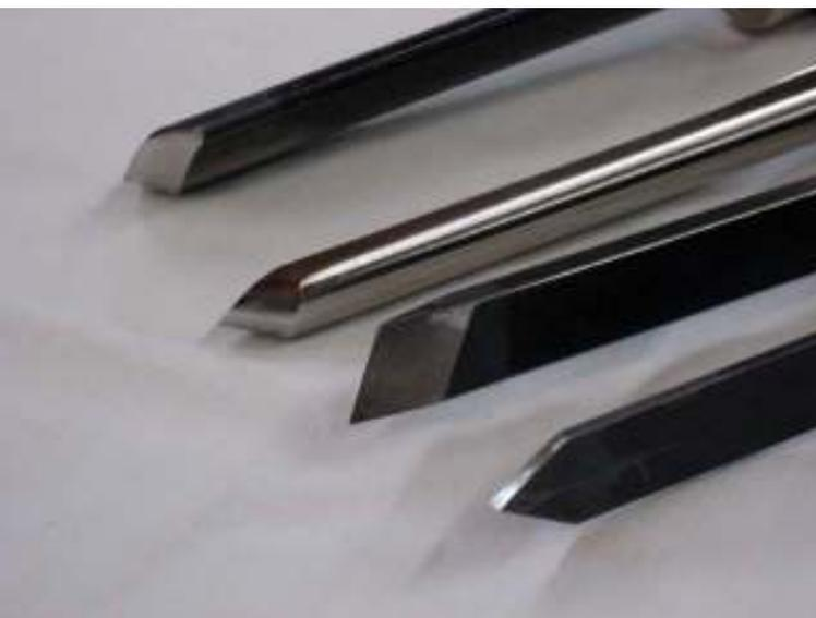
**Basic set of spindle turning tools: 1 inch spindle gouge, 1/2 inch spindle gouge, 1/2 inch skew, and parting tool. The picture on the right shows the tools rotated 90 degrees to show the grind profile which can vary quite a bit, and is less important than the sharpness of the tool. These are all cutting tools, although the skew can be used on its side as a negative rake scraper if you don't mind sharpening it often.**
