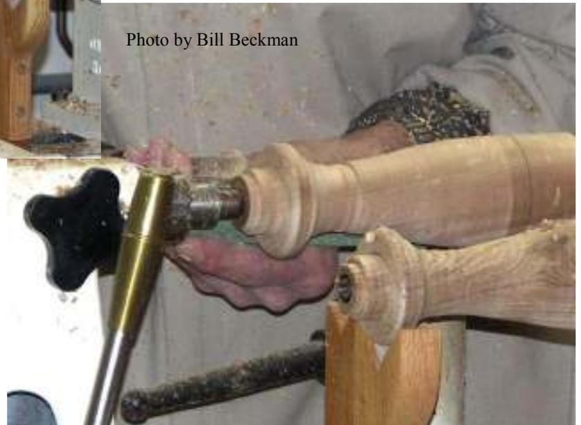
Emphasis was placed on turning precisely fitting tenons.
