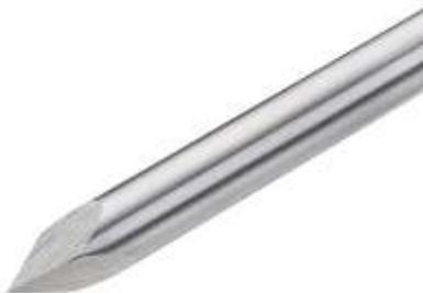
If you bring back the angle of the grind on this tool to 30 degrees or more you have a Detail Point tool that can be used to get into much smaller spaces on a finial or other turning. If used aggressively to take a larger cut this tool will be prone to catch.
