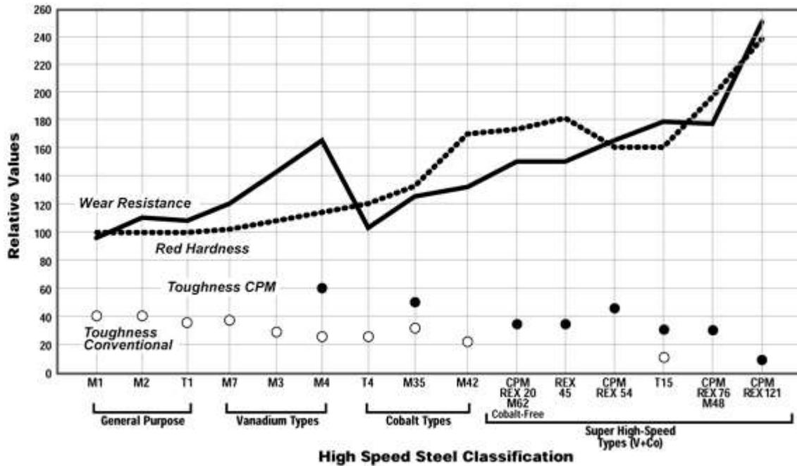
At the bottom of the chart, we have grouped the high speed steels into four major categories - general purpose (e.g. M2), wear resistant (e.g. M3 and M4), cobalt-type (e.g. M35 and M42), and super high speed (e.g. Rex 20, Rex 45, Rex 54, T15, Rex 76, and Rex 121).
