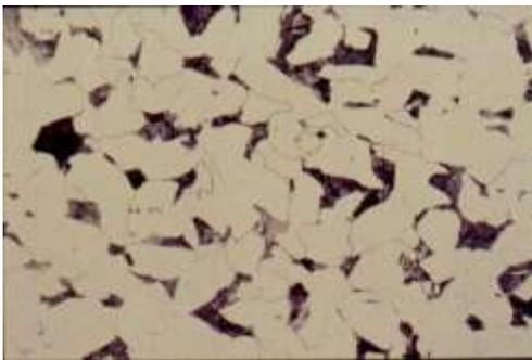
*Medium carbon steel: Approximately 0.250–0.6% carbon content. Balances ductility and strength and has good wear resistance; used for large parts, forging and automotive components.*
