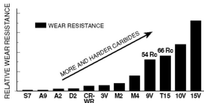
Steels with high volumes of carbide particles, or high hardness types of particles, usually exhibit the best wear resistance. Vanadium carbides, because of their hardness and chemistry, are the most effective at enhancing wear properties; chromium carbides are among the least effective.
