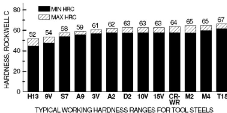
Small differences in hardness do not usually have a significant effect on the wear life of tool steels. Different tool steels are used at similar hardnesses, yet offer significant differences in expected wear life. Thus, hardness is not usually a primary factor in wear resistance, only in deformation resistance. The wear resistance of tool steels is more directly affected by their chemical composition (grade) as discussed below.
