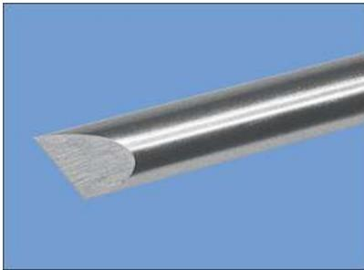
The Pyramid Point tool has three facets ground at a 45 degree angle. This is a scraper tool that can be used for layout work, to turn beads and other simple tasks. It is not prone to catches and any one of the three sides may be used as the 'up' side.
