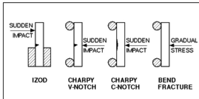
Most tool steels are notch-sensitive, meaning that any small notch present in the sample will permit it to fracture at a much lower energy. Solid carbide is even more notch-sensitive than tool steels. Thus, in addition to inherent material properties, the impact resistance of tool components is significantly impaired by notches, undercuts, geometry changes, and other common features of tools and dies.
