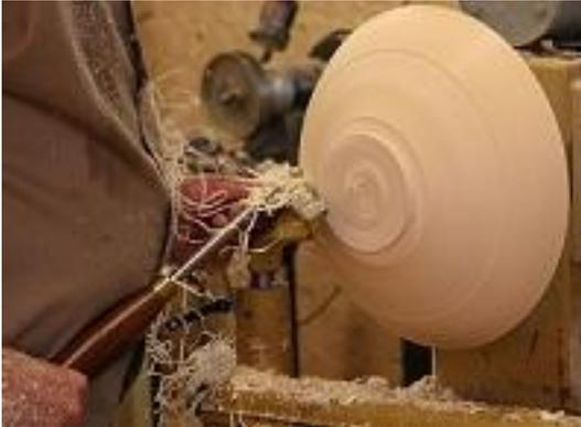
**Finishing** - page 128 – shaft horizontal, flute vertical (read warning and solution below), cut with tip opposite of the direction of the cut (left of tip used on a cut to the right), a very light cut only, catch danger on wing if too aggressive of a cut.
