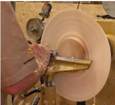
**Finishing** - shear scraping cut- page 123 - cut with edge at 45 degrees (not at 45 in this photo) to surface with lower wing, push and pull cuts, keep 'closed' flute
