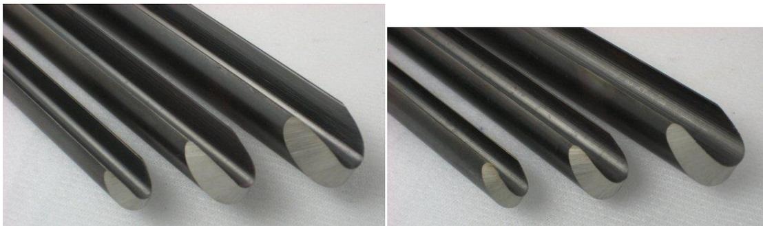
**Note: an elliptical grind adds curve to the wings of the flute and some folks like Glenn Lucas swear this is an advantage when rubbing the bevel and when scraping.**
