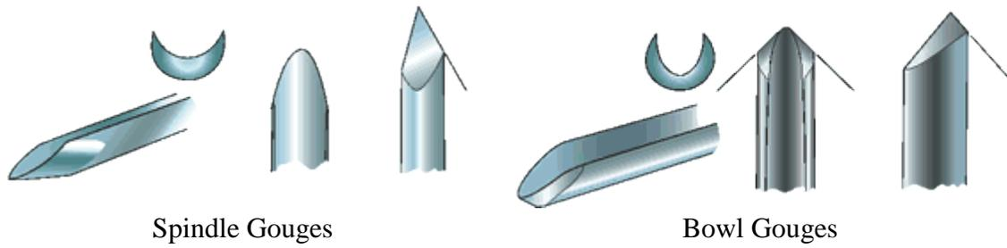
For most work, the bowl gouge will extend further over the tool rest than a spindle gouge will (as illustrated in the figures in Diagram B). This requires a heavier bar of steel with more mass to overcome or reduce vibrations.
