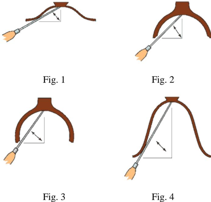
Fig. 1 – As this is a shallow type of bowl, there are no restrictions placed on the gouge by the wall of the bowl, therefore none placed on the angle of the tool.
