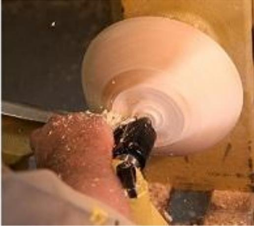
F.8 - Use the tailstock 'mark' again to re-center the bowl on the vacuum chuck (ignore for jam chuck or Cole jaws), leave the tailstock in place as long as possible for all mounting methods.
