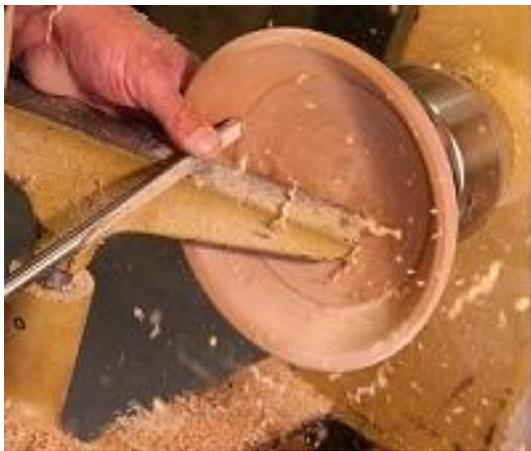
F.6 - As mentioned above, after top 1/3 of bowl is profiled grab your smaller gouge and do the finishing push cut to get the best surface. Learn to 'pick up' a new cut from where you left off with the last cut to get a smooth transition.
