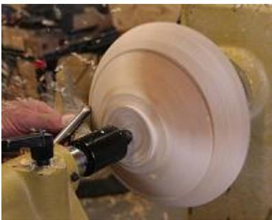
F.3 - I use a push cut to get the outside profiled as cleanly as possible. If there is no wobble on your friction mount you can do most of final profiling and finish cuts on the outside of the bowl now. Otherwise you'll have to wait until actually mounted in the chuck.
