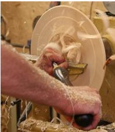
R.7 - Rough profile the inside of the bowl using a version of the roughing cut using lower wing and tip with a fairly closed flute.
