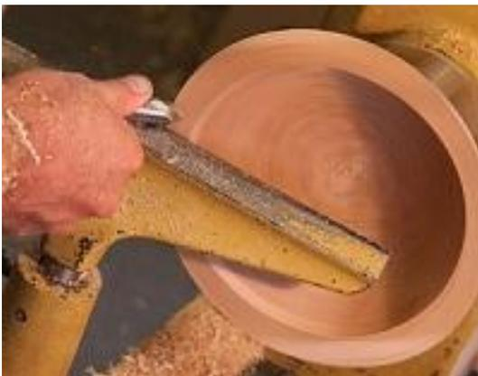
F.4 - The rim will have humped up toward pith and sagged down towards the bark. Flatten it with a shear scrape.
