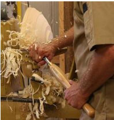
R.3 - Once the blank is basically round and you are into solid wood drop the handle, open up the flute a bit more and use the slicing cut to create the rough profile of the bowl very quickly.
