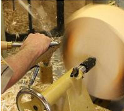
R.2 - Rough the blank to 'mostly' round using the roughing cut, shaft horizontal, flute open a bit, wing perpendicular to the axis of rotation.
