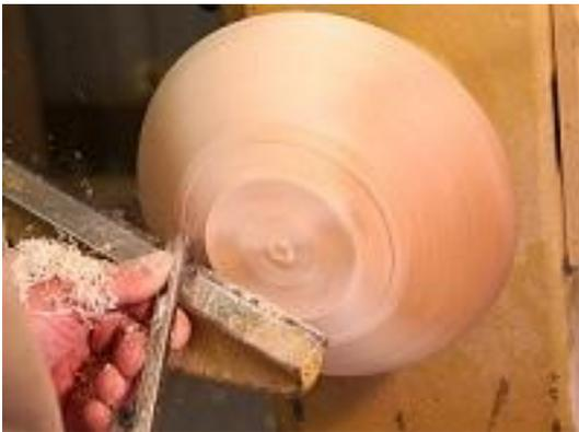
F.9 - Design your foot and transition into main body of the bowl finally turning that bottom 1/3 of the outside surface. Assume you will **not** be able to cut to the rim, make your cut fade out to nothing before you get to the section of the bowl that has warped as it almost always will during this process, shear scrape transition if needed.
