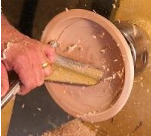
F.5 - Begin the push cut used to profile the interior of the bowl with the flute closed and then open the flute up to 45 degrees when the bevel is supported. Watch the shadow line at 4 o'clock to judge depth of cut.
