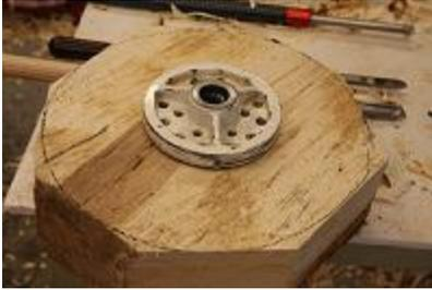
R.1 - You don't need a big band saw to cut out bowl blanks, just knock off the 'points' with your chainsaw. Don't put tailstock into bark, cut a flat with the chainsaw or chisel to get the tailstock into solid wood. I use a faceplate and larger deck screws so I can pull the tailstock away for short periods of time if necessary. I have not had much luck with screw chucks or spur drives on Minnesota's softer hardwoods.
