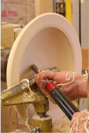
R.9 - A standard grind gouge with a steeper 60 degree bevel is handy in the bottom 1/3 of the bowl and for some types of 'difficult' grain or on very deep bowls.
