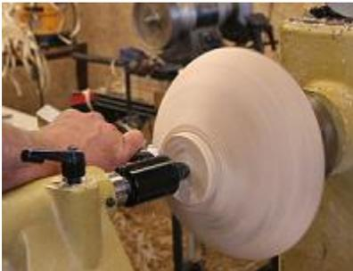
F.2 - Use the tailstock 'mark' from rough turning to re-center the bowl over the chuck.
