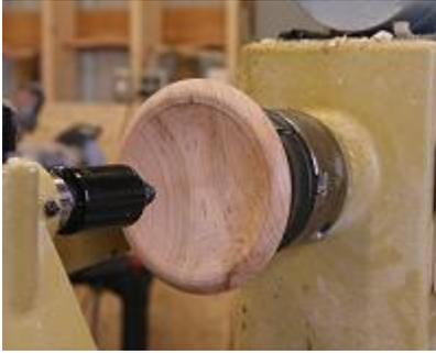
F.1 - Remounting - I use a wooden block for more diameter, better friction and to keep the metal chuck jaws from damaging the inside of the bowl.
