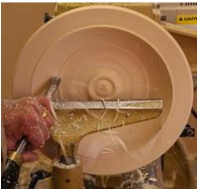
R.8 - Use a push cut to profile inside. You should be able to 'see' correct wall thickness during final profile cut if your head is positioned to left of the bowl.
