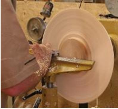
R.5 - Place blank in the chuck and use the lower wing in a scraping cut to flatten the face. Keep the flute fairly closed to avoid a catch.
