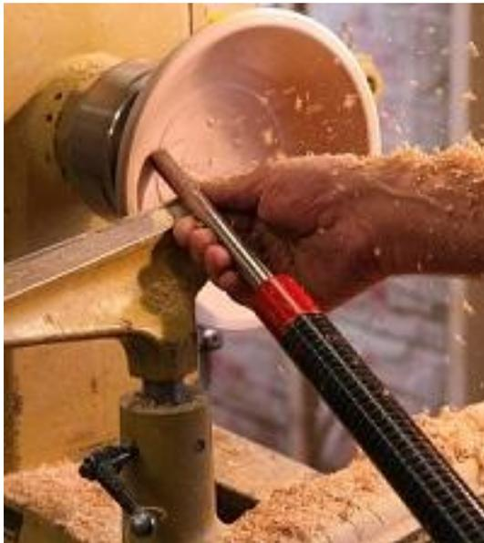
F.7 - As mentioned earlier, the bottom 1/3 of the bowl is a transition from side grain to end grain. I find a standard grind with a 60 degree or more bevel helps reduce tear out. A larger gouge (1/2 inch this case) reduces vibration when you have a lot of overhang from tool rest.
