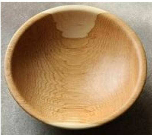
F.10 - Sanding and finishing is another demo. I try to cut cleanly enough with the tools to start with 120 grit. If 80 grit is required go easy to retain 'tool cut' look to the surface. Stay off the rim, beads and all fine edges until 180 grit. I use a 120, 180, 220 and 320 grit sequence for utility bowls.
